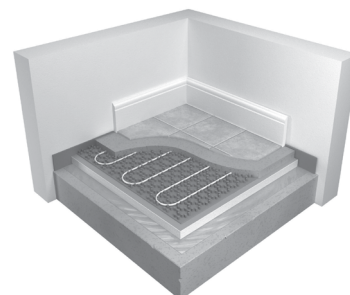
Lay the pipe
